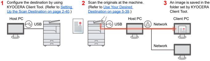
When Connecting the Machine to the PC on the Network <sup>\*1</sup>
