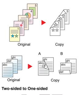
Produces two-sided copies from one-sided originals. In case of an odd number of originals, the back side of the last copy will be blank. The optional duplex unit is required.
