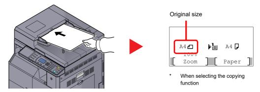
Put the side to be scanned (or the first side of two-sided originals) face-up. Slide the leading edge into the document processor as far as it will go.
